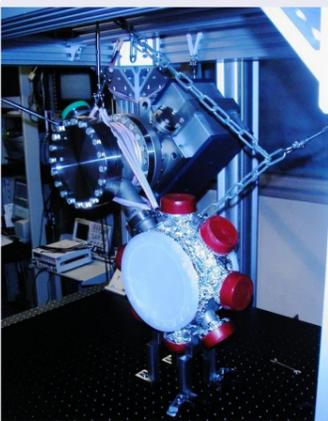
The vacuum chamber is suspended from a frame for improved optical-access.
